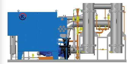
Kemco's ceramic microfiltration is a cost-effective way to achieve a high recycle rate for industries that require removal of suspended contaminants from wastewater without the addition of treatment chemicals. Through the use of ceramic elements with porosity of less than 0.1 micron, wastewater is cleansed to a recyclable quality.
